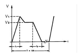
Choice of voltage:  $V_1 \le V_{peak}$  $V_2 \le V_n dc$ Maximum overvoltage ≤ V<sub>s</sub> (10 s/day)
