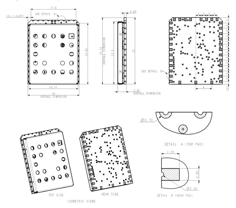
**Note:** Do not place any via or exposed pad in the inner area of the footprint to avoid short circuit between the via on customer board and the via on the bottom side of the EtherLoRa
