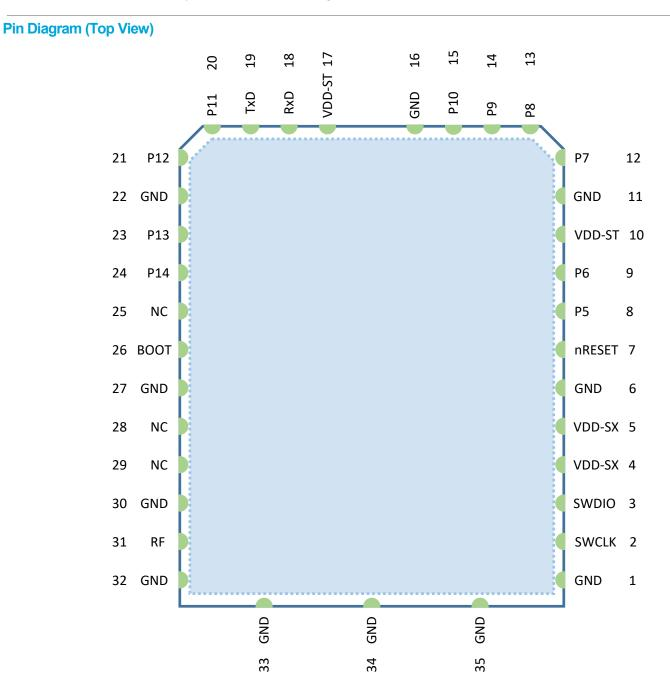
**Note:** Do not place any via or exposed pad in the inner area of the footprint to avoid short circuit between the via on customer board and the via on the bottom side of the ETH-LORA-M-AX-01
