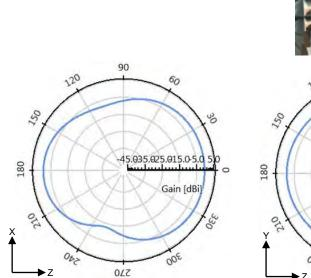
Typical performance on 40 x 100 mm PCB Measured @ 915 MHz
