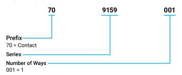
4XX 006 **Contact Description** 401 = PLUG - SMT 402 = Socket - SMT 411 = Plug - SMT - Locking **Packaging Options** 006 = Gold in Contact Area
