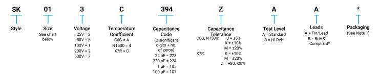
Note 1: No suffix signifies bulk packaging, which is AVX standard packaging. SK01, SK\*3, SK\*4, SK\*5, SK\*6, SK\*9 & SK\*0 are available taped and reel per EIA-468. Use suffix "TR1" if tape & reel is required.
